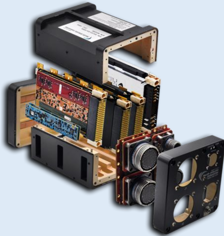
Rugged Enclosure with 38999 connectors, 3U VPX I/O cards and 3U VPX Power Supply
