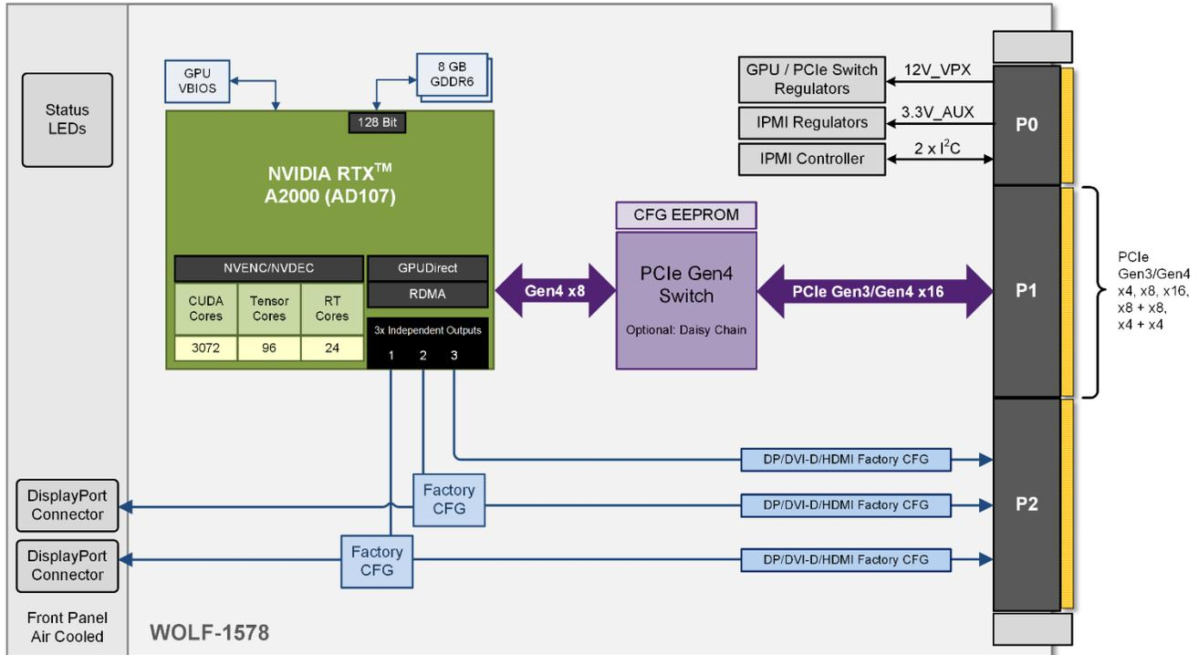
The SOSA Aligned HPC model supports slot profile 14.6.11 with PCIe supported on P1B.
