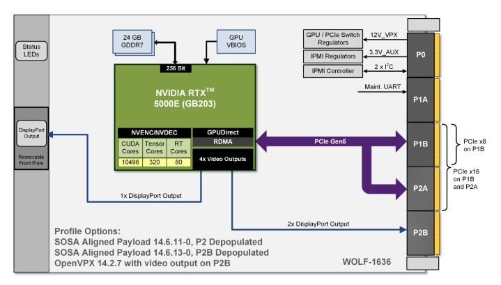
The OpenVPX profile supports DisplayPort video output, with two outputs supported on the rear connector, and one supported on the front panel under a small removeable panel. Note that the P2B pin assignment used for the video output for this product is not pin compatible with the previous generation WOLF-1538/1448/1348, for a pin compatible product see WOLF-1638.
