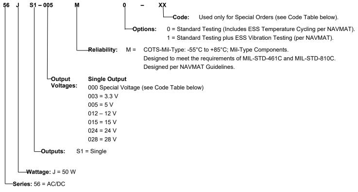
Example: 56JS1-012M0 = AC/DC; 50 Watt; Single Output; +12 V; COTS-Mil-Type; Standard Testing
