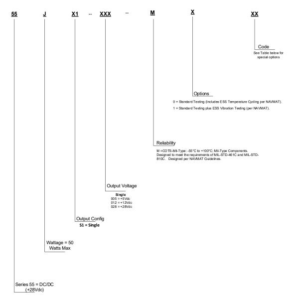
Example: 55JS1-028M0 = DC/DC (Low Voltage); 50 Watt; Single Output; +28V; COTS-MIL-Type; Standard Testing
